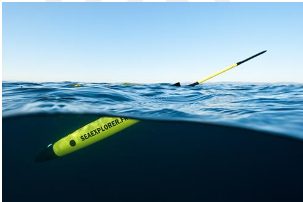
Figure 1.4 : Data transmitting and communication position of underwater glider (Autonomous Undersea Vehicle Applications Center, n.d.).
