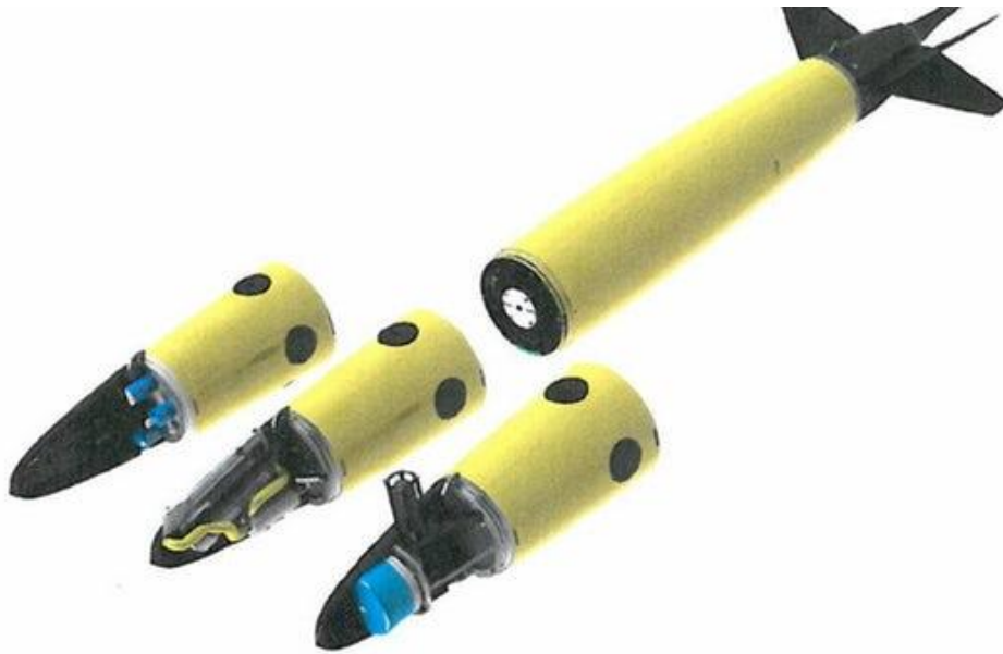
Figure 1.5 : Modular sensor payload section of an underwater glider (New Atlas, n.d.).
