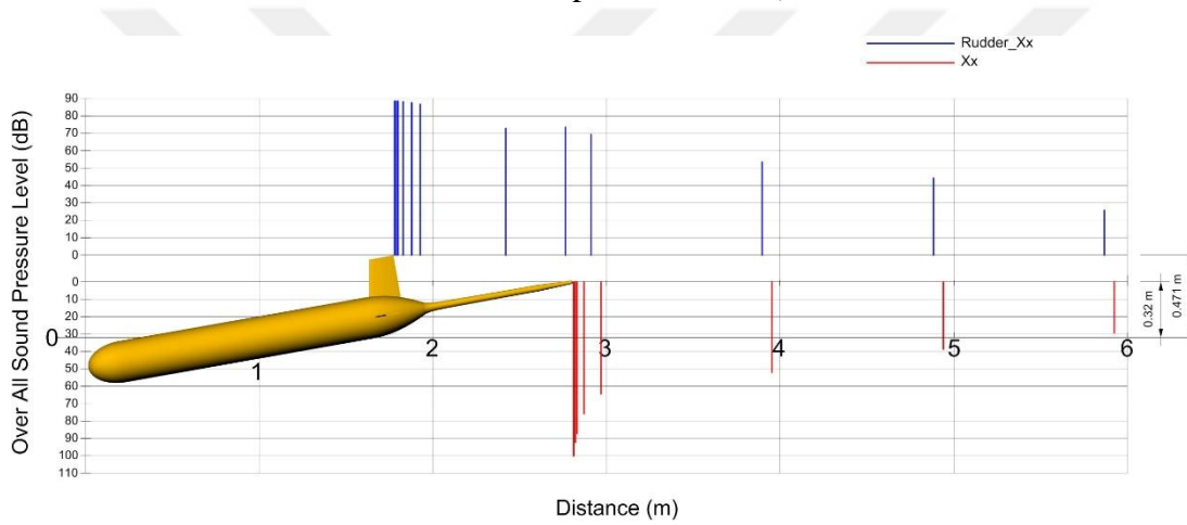
Figure 5.3 : OASPL values in XY plane for 10^\circ angle of attack case (both directions show positive values).
