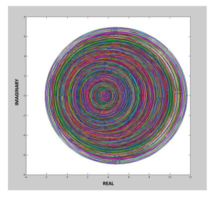
Fig. 2. Gerschgorin's circles of matrix HELM2D03LOWER\_20K
