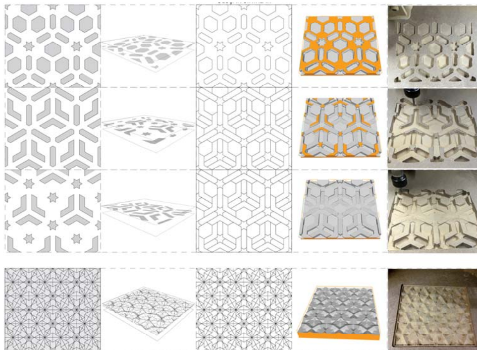
Figure 5.9 : (First three rows) Generation process of the third pattern; (Last row) Generation process of the fourth pattern.
