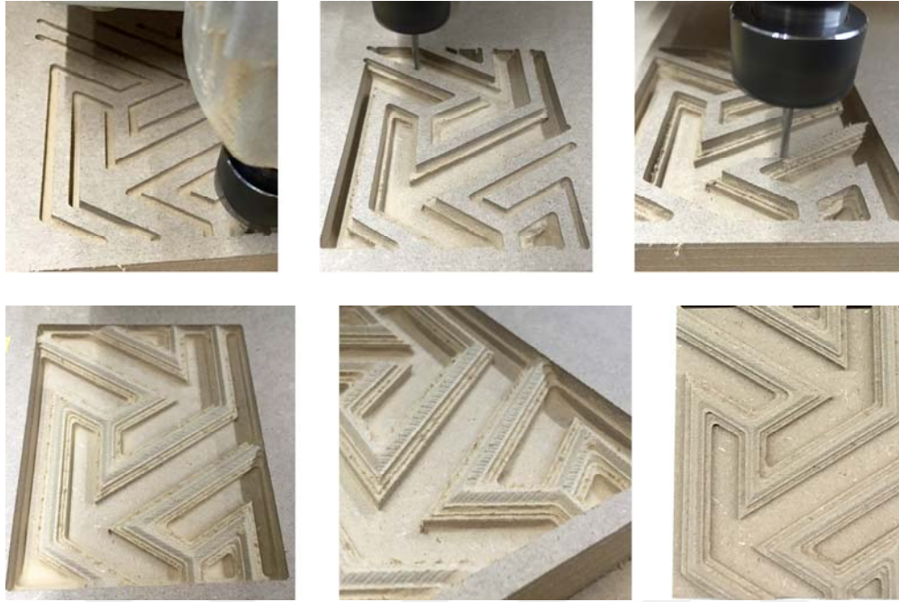
Figure 5.3 : (First row) Images of the three-phased production of Pattern I; (Second row) Images of the resulting pattern.
