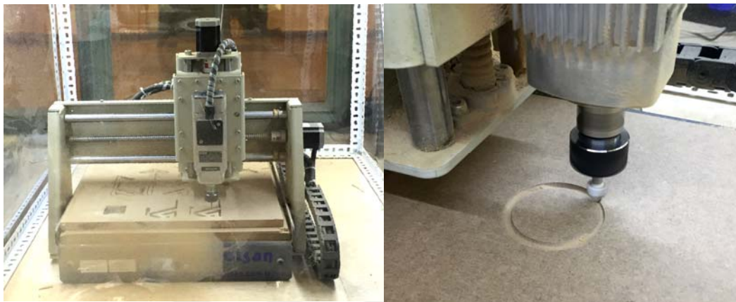
Figure 5.1 : (Left) The 3-axis CNC milling machine used in this study; (Right) Engraving through a circular path with a v-shaped milling tool.
