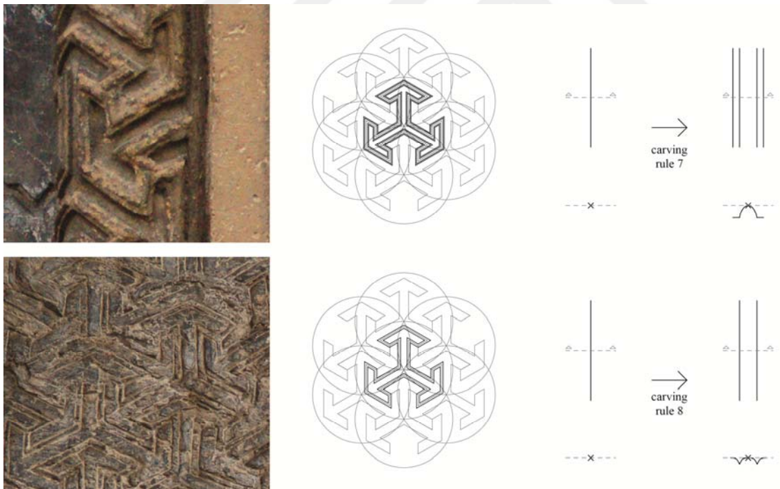
Figure 4.5 : Carving rules for generating Pattern I (first row) and Pattern II (second row) from the same initial shape.
