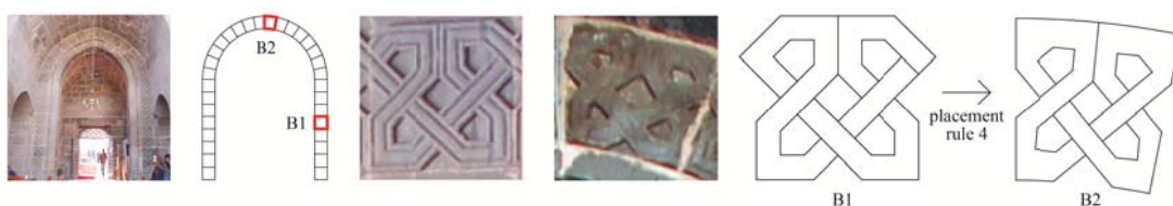
Figure 4.19 : Deformation of the geometry placed on different tiles of the arch and its placement rule formalization.
